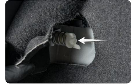
10. Remove tail lights just enough to reach between them and the body of the car. Release red clip then disconnect harness and remove tail lights. Install new tail lights in reverse order.
