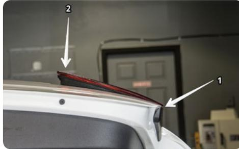
7. Secure new tail lights using OEM 8mm nuts and reconnect harnesses.
