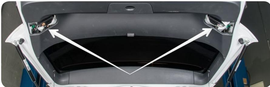
3a. Locate connectors behind the hatch lights and push red clip to unlock (1). Then push down clip (2) and unplug the harness. Remove two 8mm nuts from rear of each hatch light
