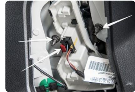
4. Using a razor blade on drivers side plug, cut off protruding tab as shown. Both sides of plug should be flat. Note: this only needs to be done on drivers side plug.
