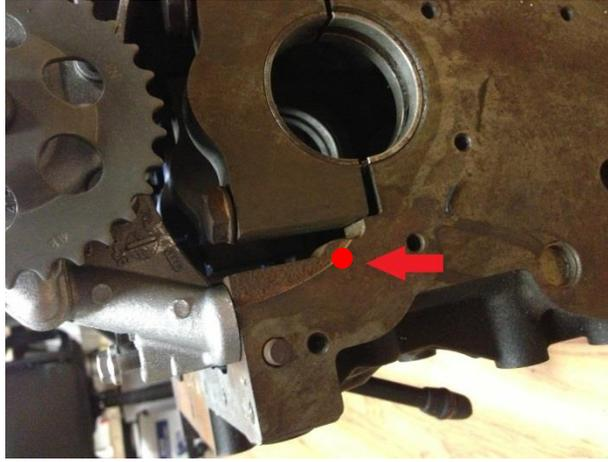
6. Heat the factory oil pump gear (on crankshaft) using a torch. When the gear is warmed up it can be removed with a 3-jaw puller. The new gear (#12) will need to be heated in an oven to approximately 300F. Once the gear is heated it will slide onto the crankshaft.
