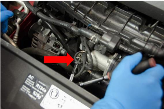
2. Remove the 7mm hose clamp securing the factory throttle body pipe to the throttle body.
