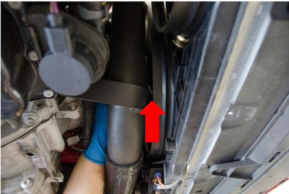
17. Check clearance between the SPULEN pipe and radiator fans. Adjust the pipe by pushing it further into the coupler if necessary.
