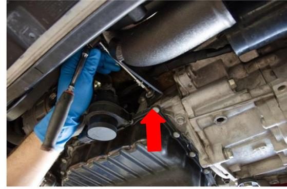
13. Install the SPULEN pipe. As you install the pipe make sure the silicone coupler goes onto the throttle body. Once installed secure the pipe with the OEM T30 torx.
