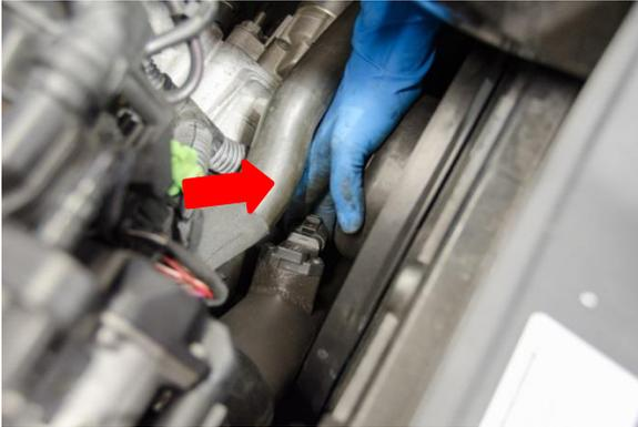
16. Reconnect the pressure sensor connector.
