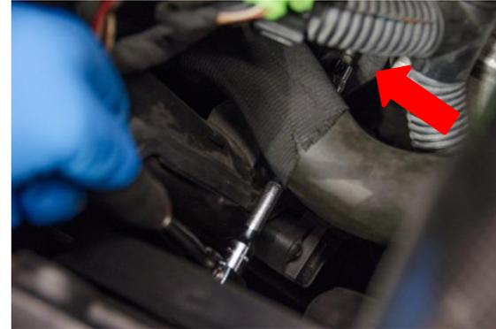
3. Remove the T-30 torx screw securing the throttle pipe.
