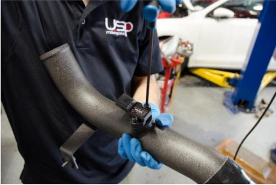
11. Install the pressure sensor into the SPULEN pipe with the connector facing downwards. Secure with the included allen head bolts.
