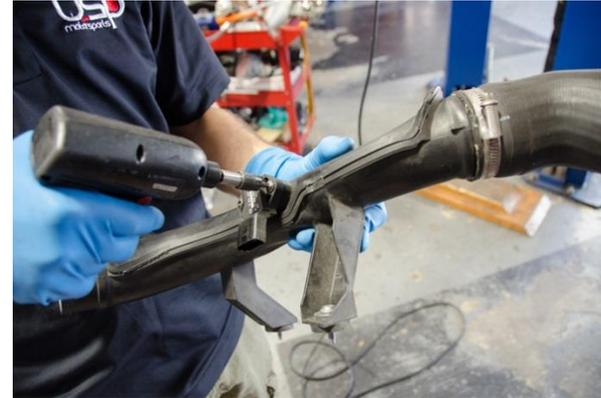
9. Remove the (2) T20 torx screws securing the pressure sensor to the throttle pipe. Remove the securing bolt and grommet.
