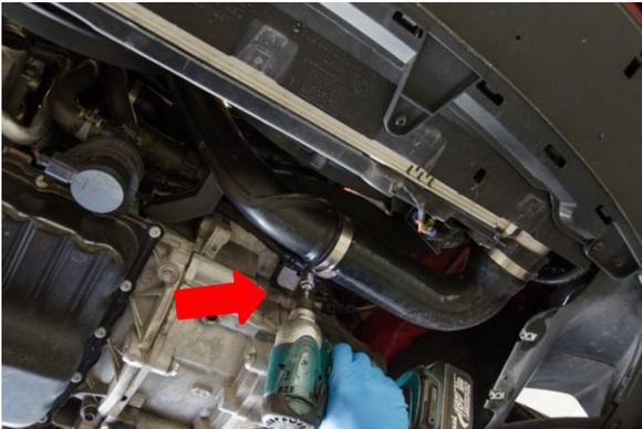
7. Using a 7mm socket remove the factory hose clamp and disconnect the rubber hose.
