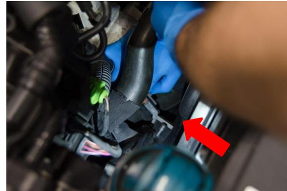
4. Disconnect the pressure sensor.
