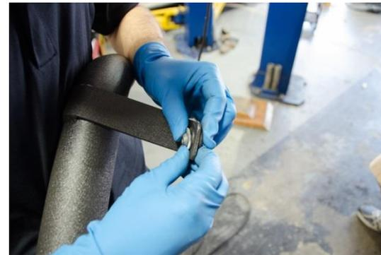
10. Install the OEM grommet and bolt into the SPULEN pipe.
