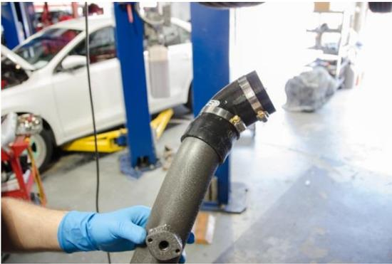
12. Install the silicone coupler and included clamps to the SPULEN pipe.
