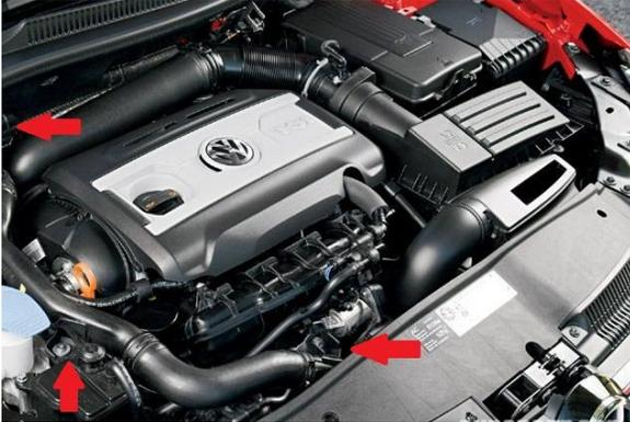
1. If your vehicle is equipped with an engine amplifier (EA) pipe remove the (2) T-30 torx screws securing the pipe. Remove the silver retaining clip located on the passenger side of the firewall by prying upwards.
