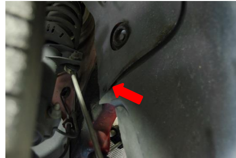
2. Remove the bottom 2 T20 torx securing the bottom fender liner followed by 5 T20 torx in the passenger wheel well. Remove the fender liner.
