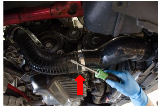
3. Remove the retaining clip and disconnect the rubber intercooler pipe.
