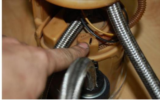
14. Take the fuel pump basket and lay it on its side inside the fuel tank. The pump assembly top will remain outside of the fuel tank.
