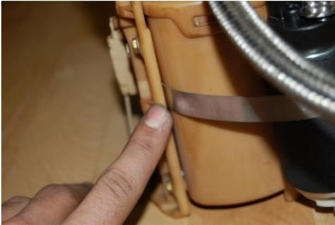
17. Place the USP fuel pump next to the factory pump basket and secure it loosely using the worm clamp. Be sure to aim the USP pump pick up towards the back of the car. This is where the mark you made on the fuel pump basket will come in handy.
