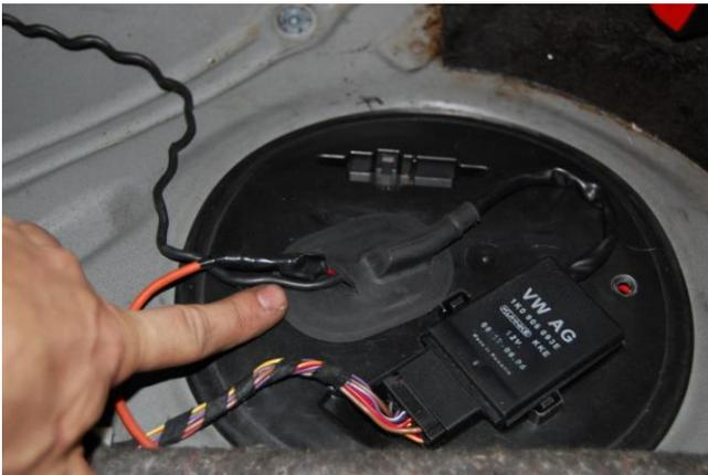
26. Connect the red power wire from the USP fuel pump and bulkhead assembly to the **red wire** from the control box and the black ground wire from the USP fuel pump and bulk head assembly to a good chassis ground.
