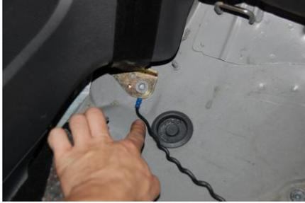
28. Route the provided red power wire around the driver side of the interior panels ending in the drivers kick panel next to the hood release.
