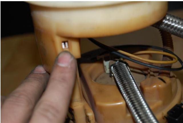
10. Take the fuel pump assembly top and drill a hole approx 5/8”.
