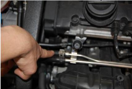
2. Using a set of pliers remove the spring clamp that secures the fuel feed line on top of the passenger side of the intake manifold. The fuel feed line is the middle black hose that has white markings on it.
