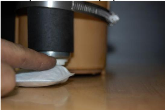
18. Once the USP fuel pump is orientated toward the back of the car and in line with the factory fuel pickup tighten the worm clamp. This is best done using a skew driver or 90 degree bit attachment. Although, it can be done with a 1/4" ratchet.
